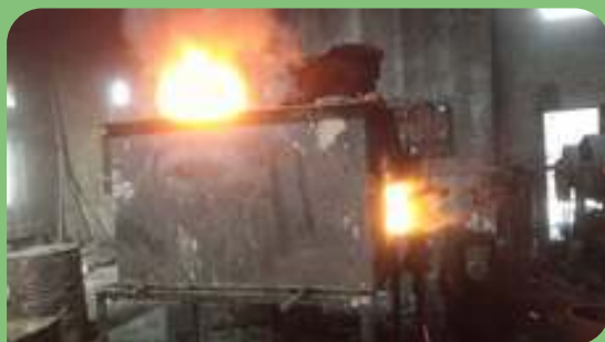
Figure 8: Conventional forging furnace
