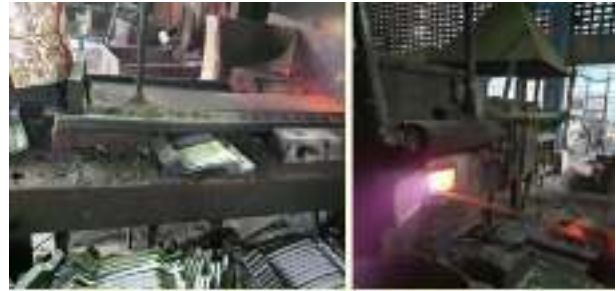
Figure 3: Conventional furnace oil fired forging furnace in Ludhiana hand-tool cluster
