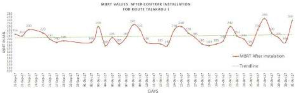
Figure 31: MBRT after installation of remote monitoring system
