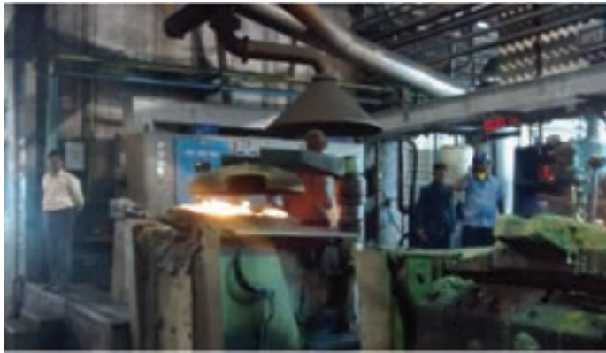
Figure 12: Induction Furnace Lid Mechanism
