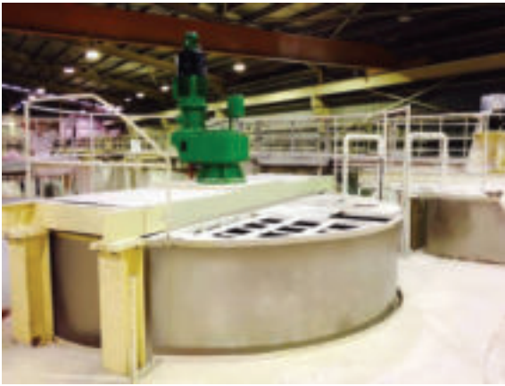
Figure 6: Slip agitation and storage
