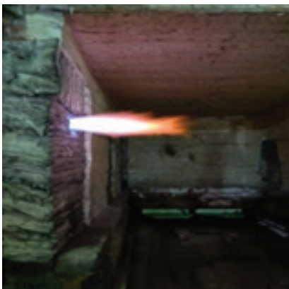
Figure 67: High Velocity Burner with Flame
