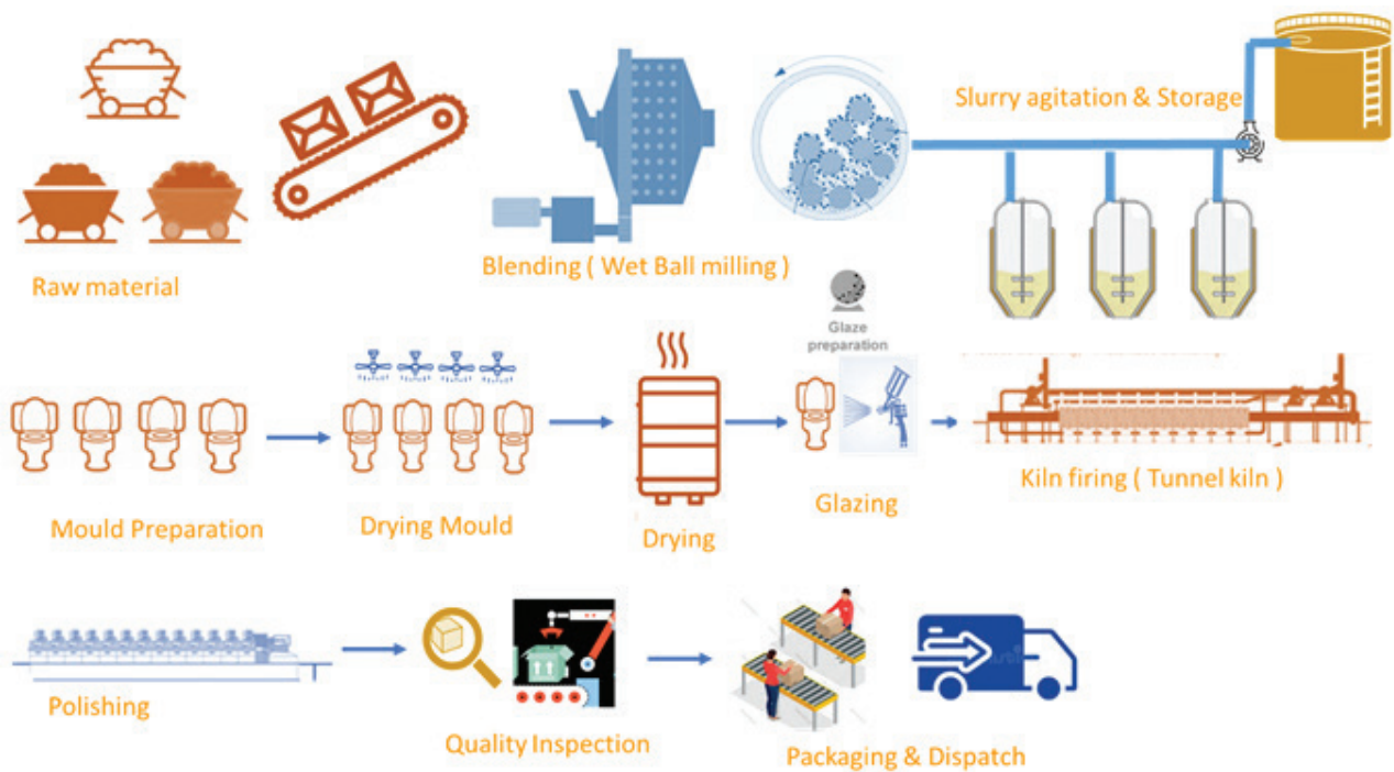
Figure 13: Ceramic Sanitaryware Manufacturing Process Flow
