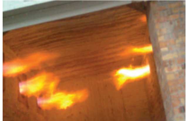
Figure 69: Improper air to fuel ratio
