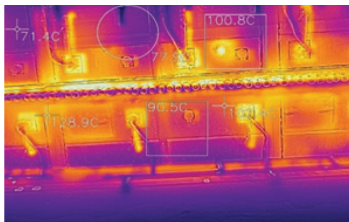
Figure 32: Surface temperature at firing zone in a kiln
