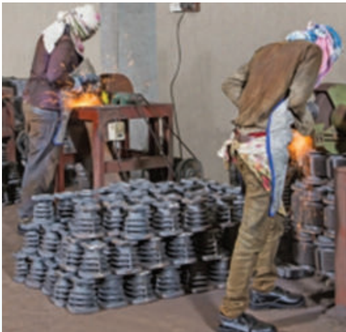
Figure 43: Grinders in foundry
