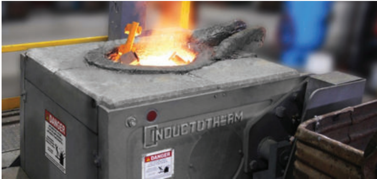
Figure 17: Induction furnace without lid mechanism
