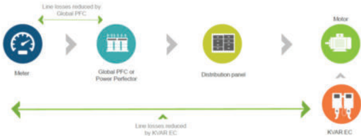
Figure 36: Operation of kVAR compensator
