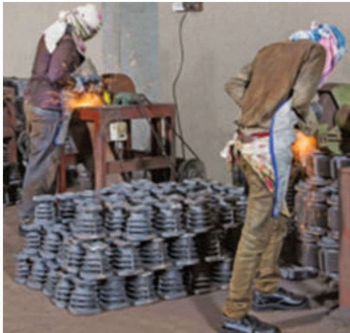
Figure 47: Use of electric grinders in place of pneumatic grinders
