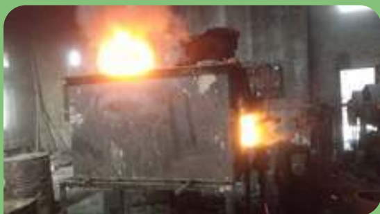
Figure 8: Conventional forging furnace
