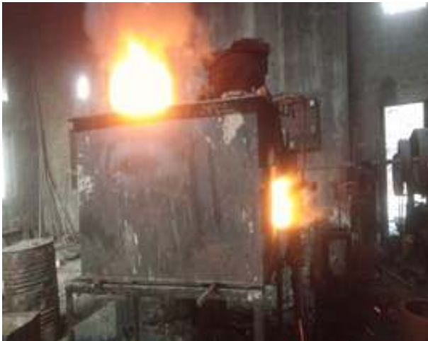
Figure 4: Conventional furnace oil fired forging furnace
