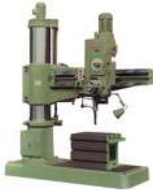
Figure 7: A conventional drilling machine
