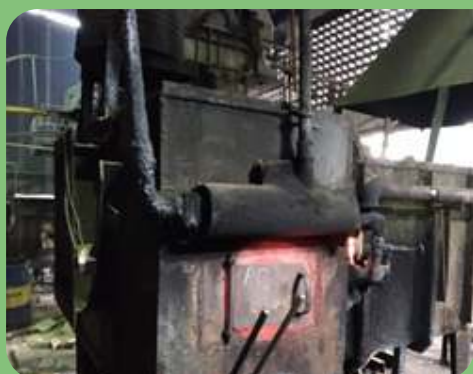
Conventional FO Fired Forging Furnace
