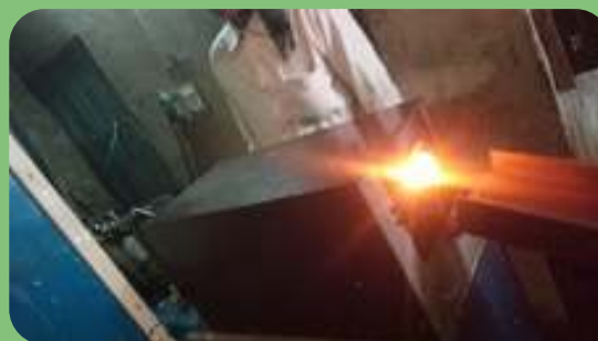
Electric Induction Billet Heater at Kohinoor Forging
