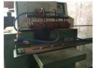
Figure 14: An induction billet heater
