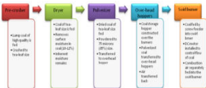
Figure 19: Process flow of pulverized coal handling and feeding system
