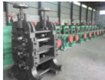
Figure 28: Roller bearing based mill stand
