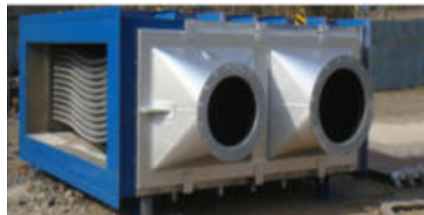
Figure 14: Cross-flow U-tube type metallic recuperator
