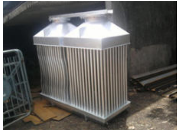
Figure 11: High efficiency metallic recuperator
