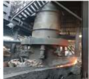
Figure 5: Single blast cupola
