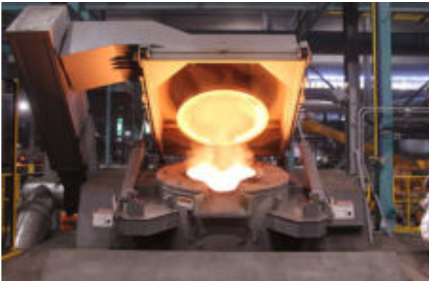
Figure 19: Lid Mechanism in an Induction Furnace
