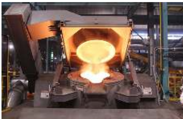
Figure 19: Lid Mechanism in an Induction Furnace
