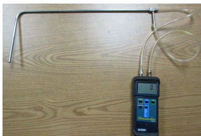
Figure 39: Pitot Tubes (and Digital Manometer) used in a Steam System Assessment
