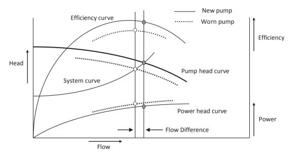
Fig. 6.6. Effect of worn pump on pump characteristics
