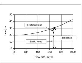
Fig. 4.3. System Curve Components
