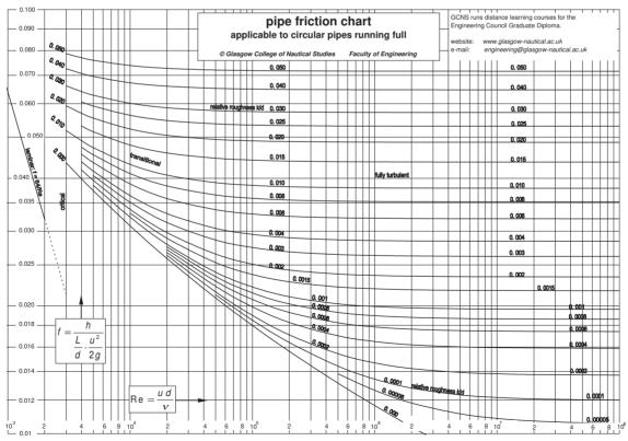
Fig. 4.1. Moody diagram for pipe losses
