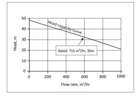
Fig. 5.1. Centrifugal pump head capacity curve
