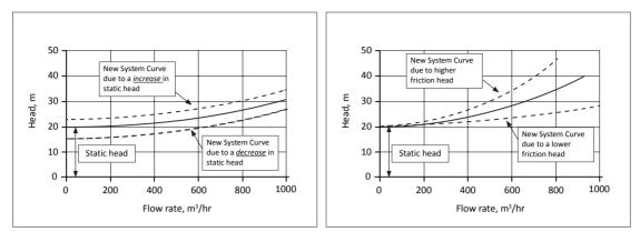
Fig. 4.4. Impact of static head changes on system curve
