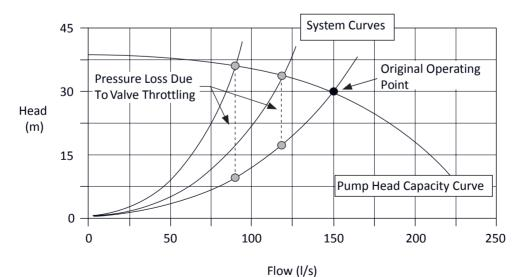
Fig. 9.2. Throttling of a centrifugal pump.
