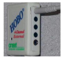
Fig. 12.32. General Purpose Data Logger
