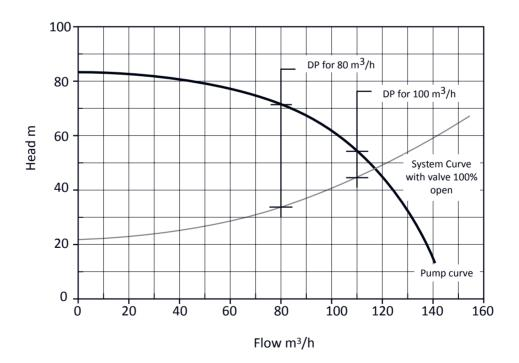
Fig. 14.2. Pump and system curves
