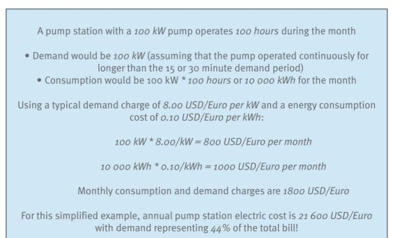
The above example shows that the impact of demand charges that must be accounted for to maximize energy cost savings when pump systems are optimized.
