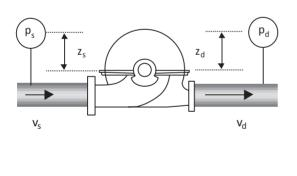
$$H_{p} = \left(\frac{V_{d}^{2} - V_{s}^{2}}{2g}\right) + \frac{2.31}{s.g.}(p_{d} - p_{s}) + (z_{d} - z_{s})$$
