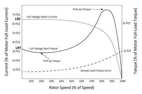
Fig. 8.2. Typical torque-speed curve for a 3-phase AC induction motor
