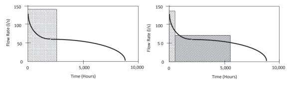
Fig. 2.6. Flow duration diagram for a large wastewater pump
