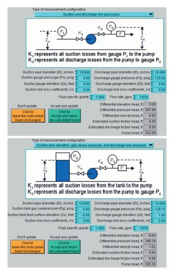
Fig. 12.17. Taps for Measuring Suction and Discharge Pressure
