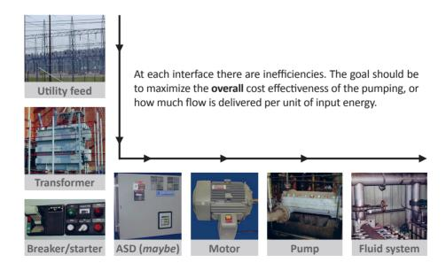
Fig. 2.1. System components
