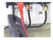
Fig. 12.28. Monitoring all Three Phases
