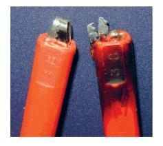
Fig. 12.25. Normal and Vaporized Test Lead
