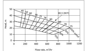
Fig. 5.3. Pump curves for varying speeds
