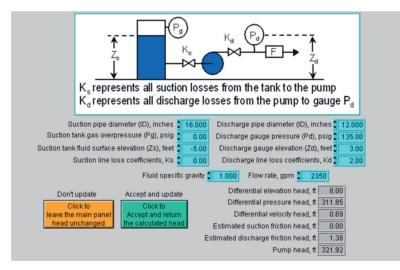
Fig. 12.11. Pump head Calculator W/ Component Loss Calculator
