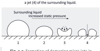
Cavitation bubble imploding close to a fixed surface generating
