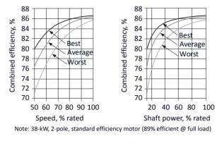
**Fig. 7.3.** Combined motor / drive efficiency when attached to different drives, (DOE)
