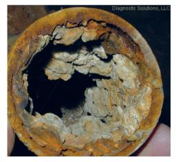
Fig. 4.2. Water distribution pipe with significant tuberculation (courtesy of Diagnostic Solutions)
