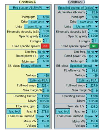
Fig. 15.2. PSAT input section
