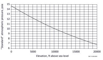
**Fig. 12.4.** Atmospheric Pressure as a Function of Elevation
