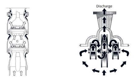
Fig. 3.6. Vertical and horizontal multistage pumps
