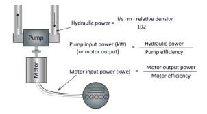
Fig. 7.1. Breakdown of Energy Equation
