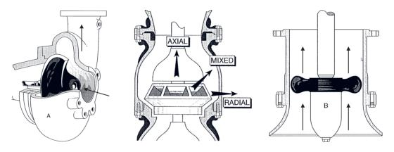
Fig. 3.5. Centrifugal pump flow patterns (radial, mixed and axial)
