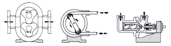
**Fig. 3.8.** Examples of Rotary Lobe, Tube and Screw Pumps *(Figures courtesy of Hydraulic Institute)*
