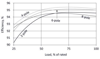
Fig. 8.3. Typical efficiencies for 60Hz, 75 kW motors
