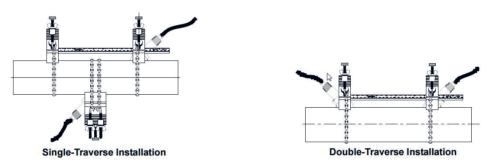
**Fig. 12.23.** Single and Double Traverse Methods (courtesy of GE Panametrics)
