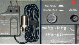
Fig. 12.14. Inaccurate Pressure Gauge and PV-350 Pressure Indicator
