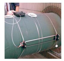
Fig. 12.22. Transit-time ultrasonic flow meter
