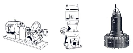
Fig. 3.4. Frame mounted and close coupled pumps
