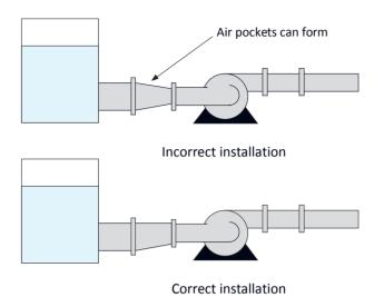
Fig. 6.1. Suction pipe installation
