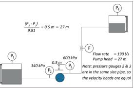
Fig. 13.3. Calculating friction head
