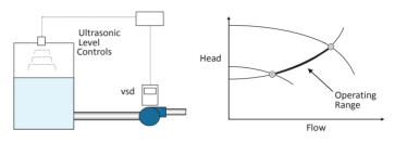
Fig. 9.10. Level controls using a vsd equipped pump
