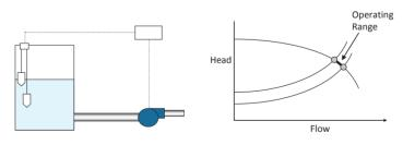
Fig. 9.9. On/off level control
