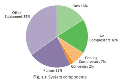
The large amounts of energy used for pumping makes pump systems a major candidate for energy savings. Of the energy used for pumping, about 75% is used for centrifugal pumps and the remaining 25% for positive displacement pumps.
