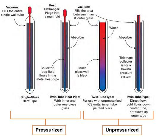
Figure 26 Heat pipe breakdown components
