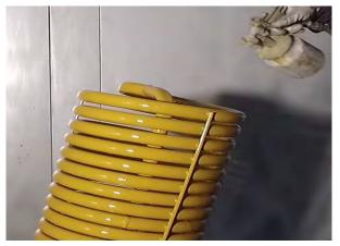
Figure 87 Heat exchanger tubes outer coating [10]
