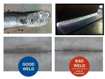
Figure 58 Difference between good and bad welding upper and lower sides [I-car.com/welding]
