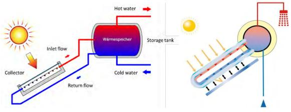
Figure 7 Functional diagram of a Thermosiphon open systems [1]
