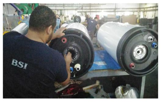
Figure 79 Seal joint fixing [3]
