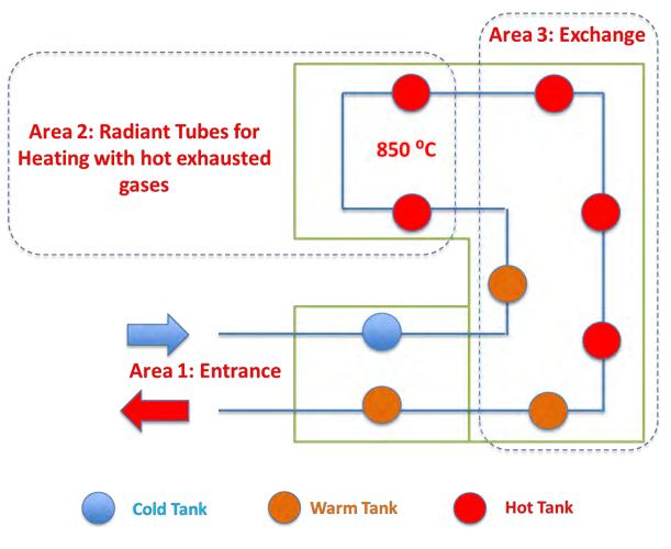
Figure 69 Enamel coating firing process of tanks
