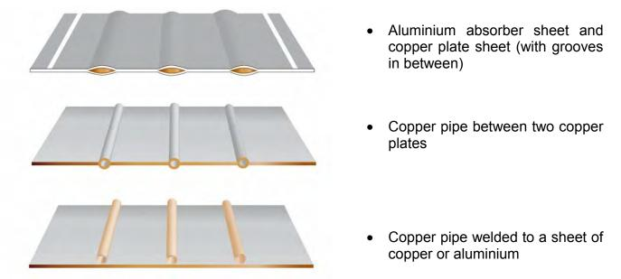
Figure 91 Different absorber configurations [3]
