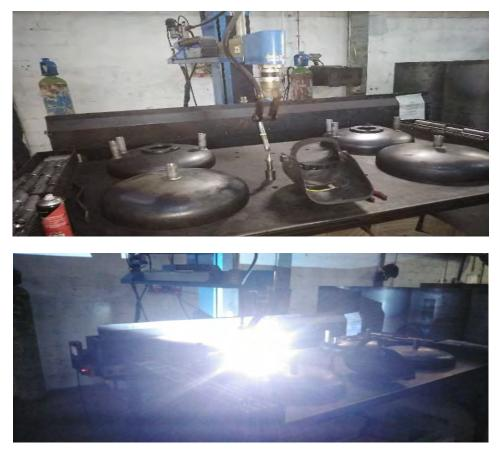
Figure 52 Robotic arc welding of pipe connections to dished heads [3]
