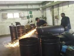
Figure 54 Tack welding and surface cleaning of the circular surface [3]
