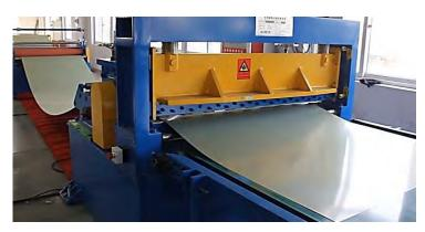
Figure 42 Inner tank sheet cutting [3]
