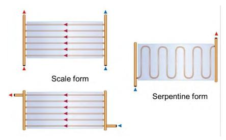
Figure 92 Absorber grid form types [3]
