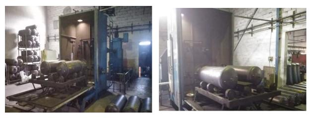
Figure 62 Inner tank sand blasting process (preparation and loading) [3]
