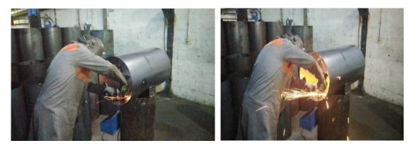
Figure 48 Linear welding treatment [3]
