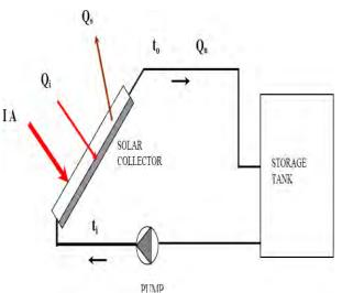
Figure 19 SWH system schematic diagram
