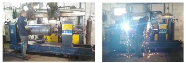
Figure 55 Circular welding using Automatic MIG welding machine [3]
