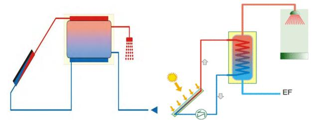
Figure 8 Functional diagram of thermosiphon closed systems
