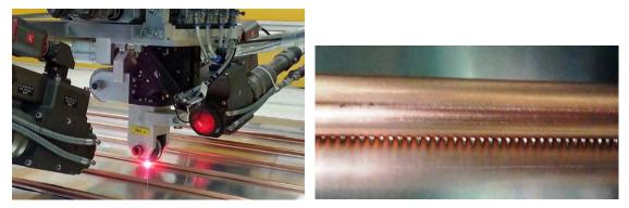
Figure 105 Laser welding of riser tubes and absorber sheet [4]
