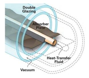
Figure 25 Heat pipe breakdown components
