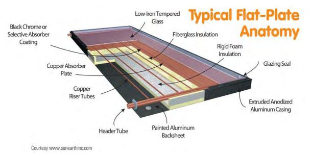
Figure 23 Flat plate collector typical breakdown components [9]
