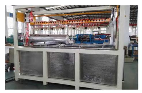
Figure 60 Water bath for leakage test using compressed air
