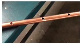
Figure 97 Punched holes along header tube length [4]
