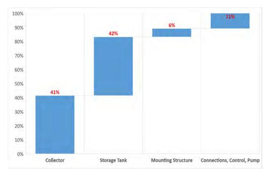
Figure 32 SWH system cost breakdown [1]
