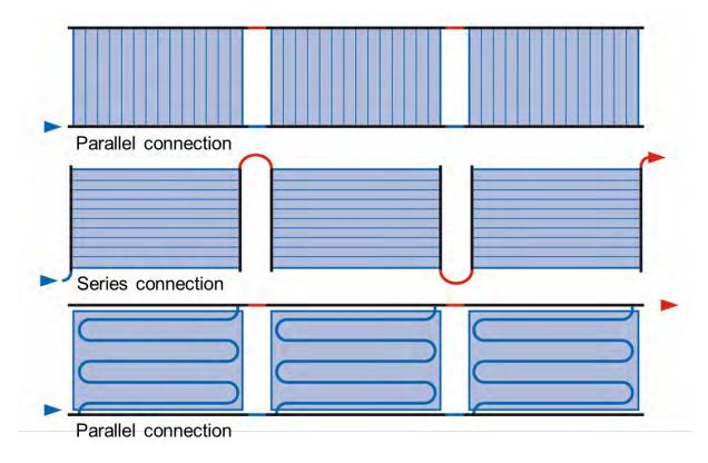
Figure 93 Absorber types of connections [3]
