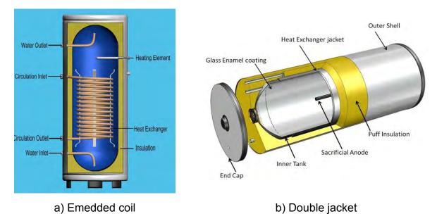
Figure 22 SWH storage tank different configurations
