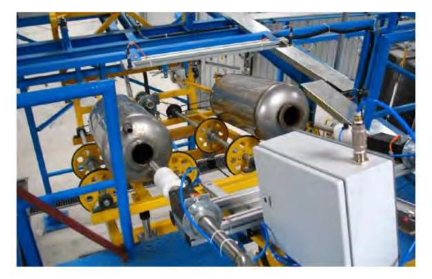
Figure 67 Enamel coating injection process (Flooding) [7]
