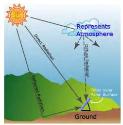
Figure 2 Type of solar radiation
