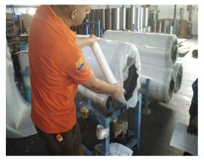
Figure 83 Packaging of SWH storage tank
