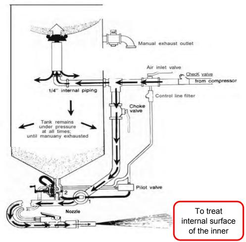
Figure 61 Schematic diagram of portable sand blasting machine [6]
