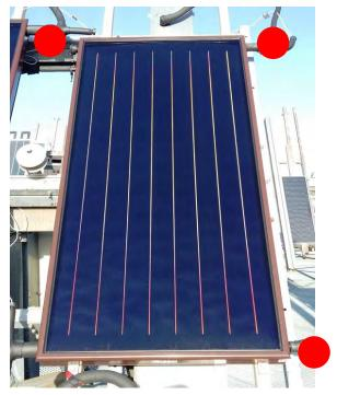
Figure 129 Exposure test for flat plate collector [11]
