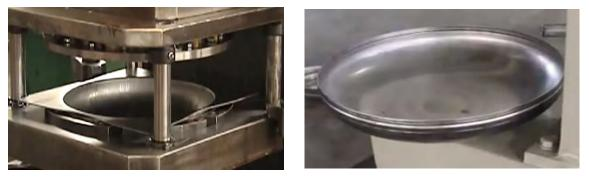
Figure 50 Rounding of inner tank end covers by used of piston
