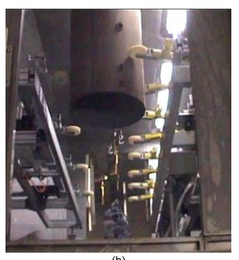
(a) (b) Figure 68 Enamel coating by (a) powder and (b) spray<sup>6</sup>
