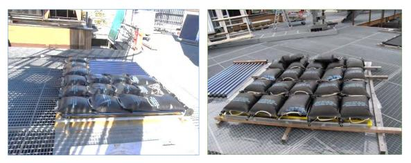
Figure 131 Mechanical load testing [11]
