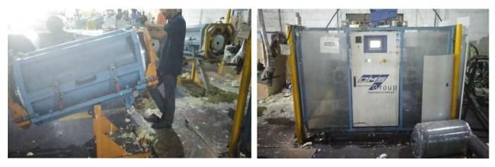
Figure 78 Foam insulation injection machine [3]
