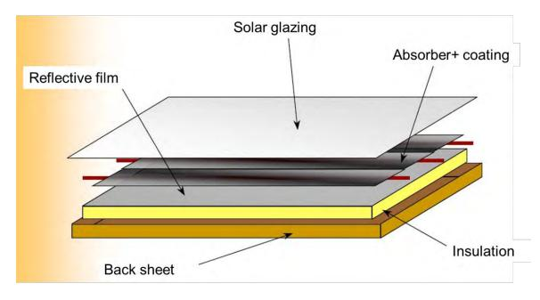
Figure 90 Flat plate collector main components [3]
