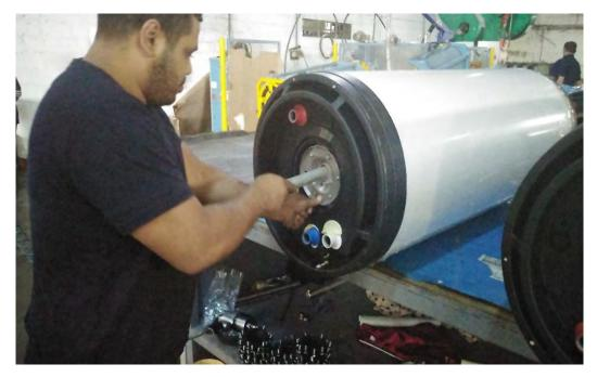
Figure 81 Mg rod fixing [3]
