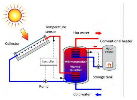
Figure 9 Functional diagram of a forced circulation system [1]
