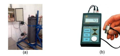
Figure 73 Enamel coating thickness testing (a) dielectric intensity and (b) ultrasonic thickness detector
