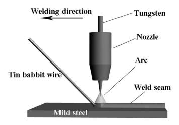
Figure 47 Schematic diagram of arc welding [5]
