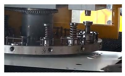
Figure 43 Ports punching in tank body [4]
