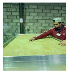
Figure 107 Insulation placement inside the frame casing [3]
