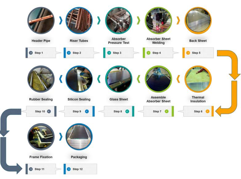
Figure 95 Flow chart of flat plate collector manufacturing process
