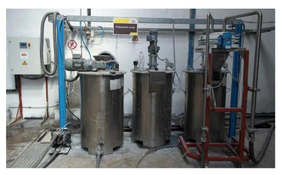
Figure 64 enamel coating preparation mixing unit [3]
