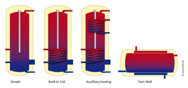
Figure 39 Different storage tank configurations
