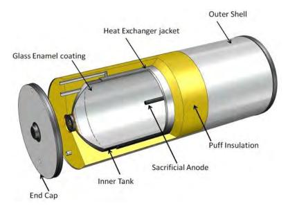
Figure 88 Sample of double jacket storage tank
