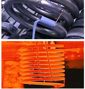
Figure 86 Heat exchanger tube inner coating
