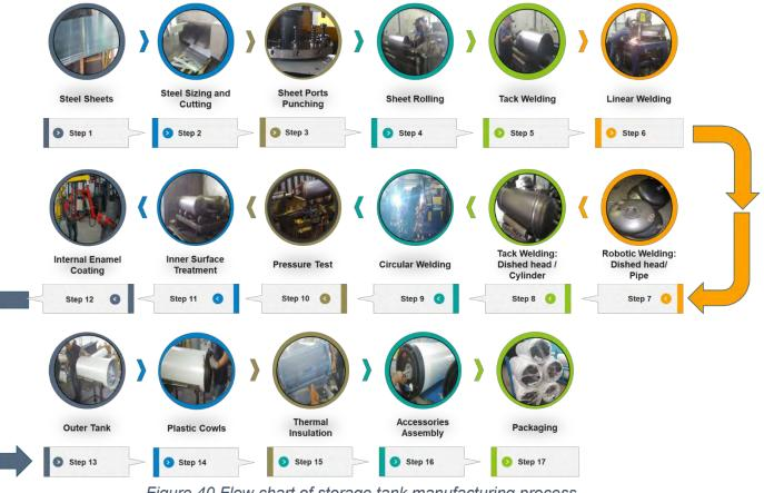
Figure 40 Flow chart of storage tank manufacturing process
