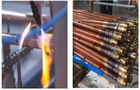
Figure 98 Header tube fitted with connection joints [4]
