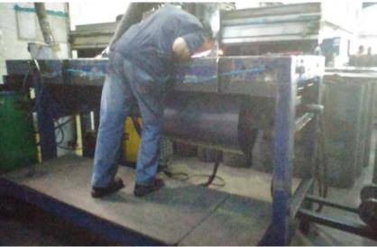
Figure 46 Linear welding of inner tank [3]
