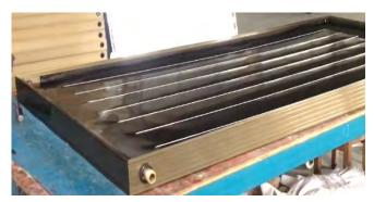
Figure 108 Absorber plate and frame assembly
