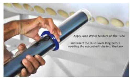
Figure 118 Assembly of evacuated tube with storage tank
