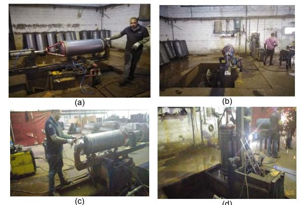
(C) (d) Figure 59 Pressure test steps for the inner tank (a) tank fixation, (b) tank filling with water, (c) installation of pressure gauge, (d) empty tank of water [3]
