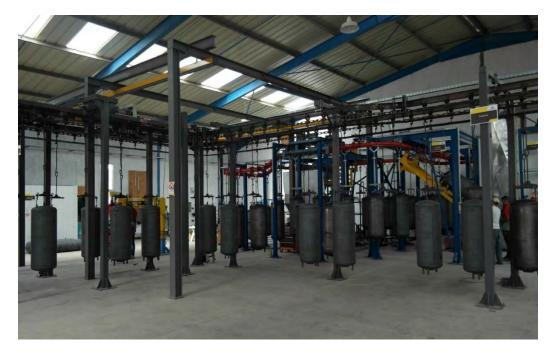
Figure 71 Enamel coated tanks cooling process [3]
