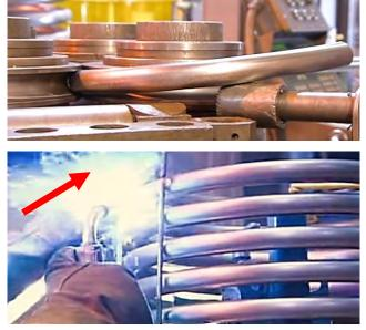
Figure 85 Heat exchanger coiling
