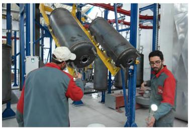
Figure 74 Visual inspection of internal enamel coating [3]
