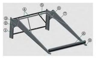
Figure 119 Main parts of the mounting structure
